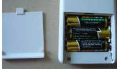
Remote is powered by three pcs AA Dry-cell. When the LCD shows “Battery Low”, please change batteries. Please power off and take out batteries if long time not using.
